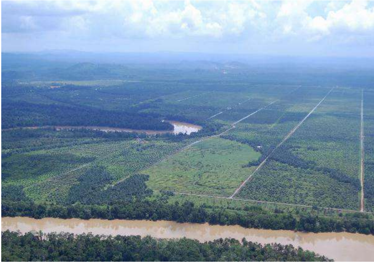
Figure 3.1 Roads and drainage channels should, as far as possible, be located outside riparian reserves to reduce gaps along the riparian reserves, and also to prevent water from oil palm plantations sidestepping the riparian reserve vegetation and flowing directly into natural waterways. Photo: HUTAN/Marc Ancrenaz.
