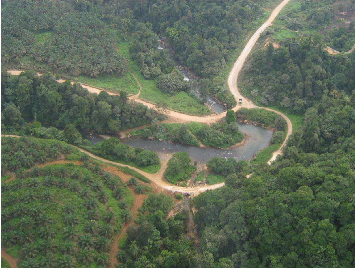
Figure 2.3 Gaps in riparian reserves, including roads and/or small streams and drainage channels without riparian reserves, enable pollutants to enter natural waterways, bypassing the filtration mechanism of riparian reserve vegetation. Gaps along the lengths of riparian reserves should therefore be minimised as far as possible, while small waterways should be managed carefully to minimise the movements of pesticides, fertilisers and sediments into larger waterways (see Section 2.1.1). Photo: C. Beamish/Wilmar.
